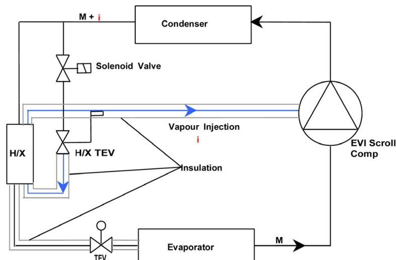
Figure 3-2: Vapour injection
