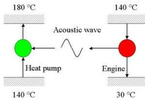
Figure 3-7: Thermo acoustic heat pump
