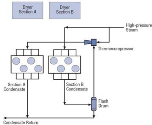
Figure 3-6: Thermal vapor recompression, Example from Japan
